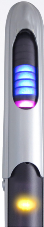
Located the ferrous hazard with amber lights in column
